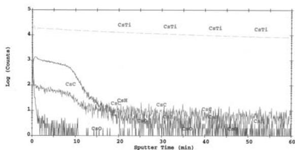
Fig.1 Depth profile of a surface layer in titanium as abraded.
