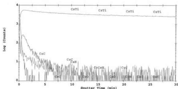
Fig.4 Depth profiles of surface annealed at 100°C in air, followed by exposure to ozone at 150°C.
