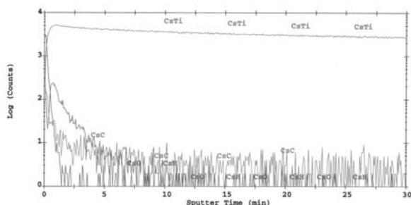
Fig.5 Depth profiles of surface annealed at 150°C in air, followed by exposure to ozone at 150°C.
